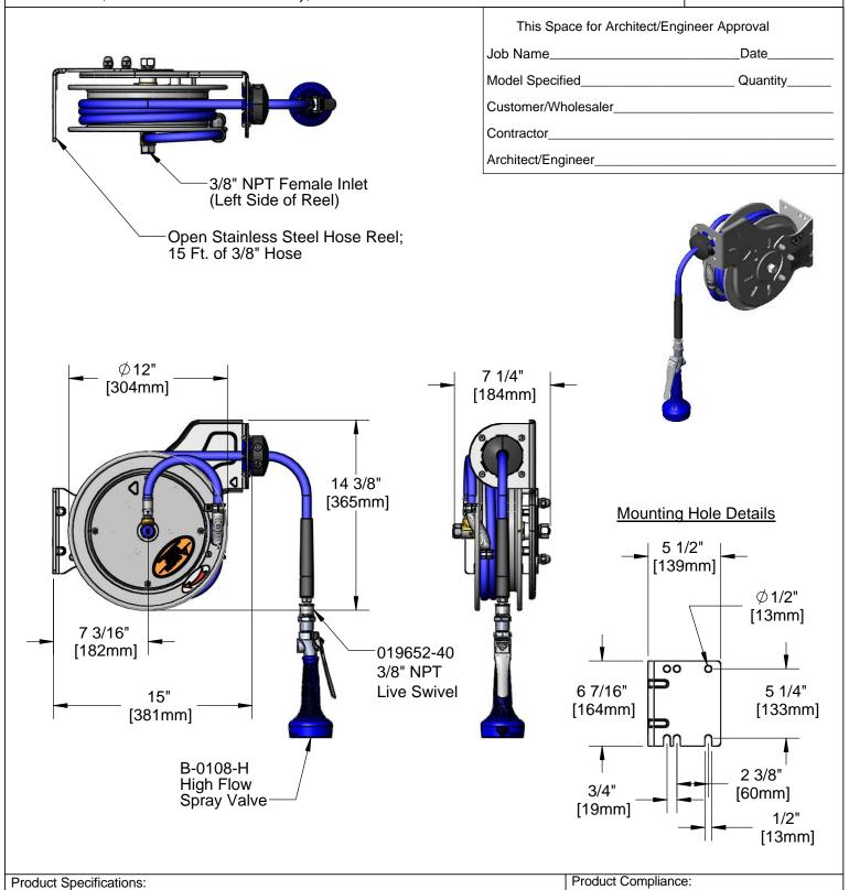
3/8" x 15 Ft. Open Stainless Steel Reel with High Flow Spray Valve & Swivel
